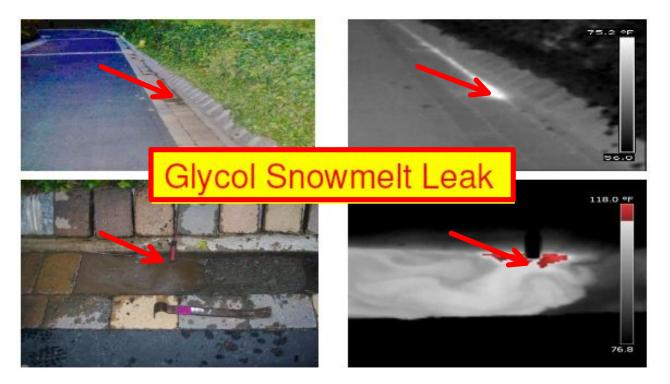
Infrared thermal imaging detected the hot leaking glycol which is visible in the photos and thermograms. The origin of the leak was detected at the hottest spot. The use of infrared saved the repair contractor approximately 2.5 hours of labor and needless destructive testing.
