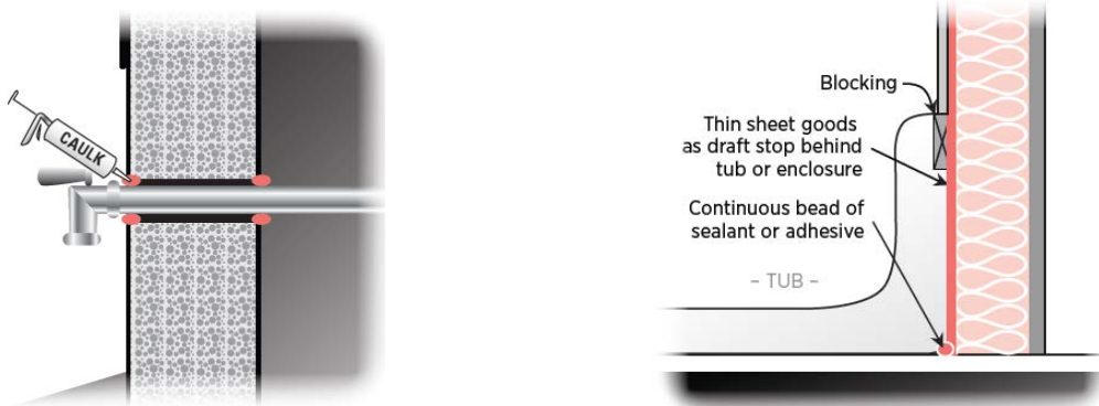
Above left: Caulk all plumbing penetrations through exterior walls.
