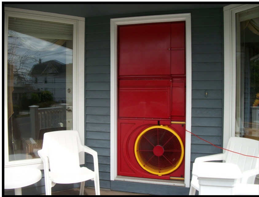
Blower door engaged to depressurize residence and simulate wind storm activity.
