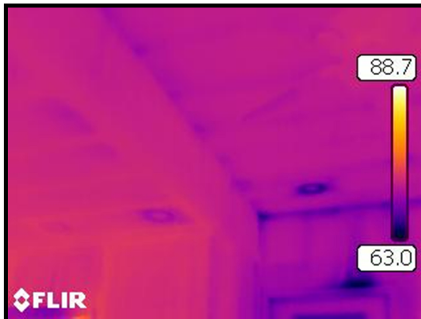
Thermograph taken before beginning applying moisture via the spray rack and engaging the blower door fan.
